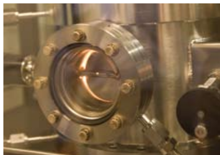
A metalorganic chemical vapor deposition reactor deposits nanostructures one atomic layer at a time on a semiconductor wafer.
